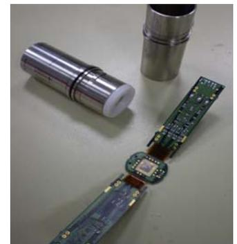
Fig. 2: Complete and disassembled TAS with PCB and  $\mu$ C
