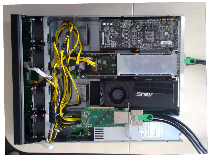
PCIe 2.0 Extension Box with 4 GPU adapters
